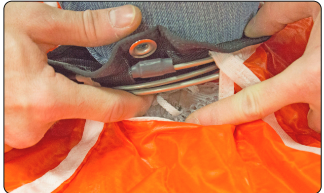
10.15 Folding and stowing the center line.
