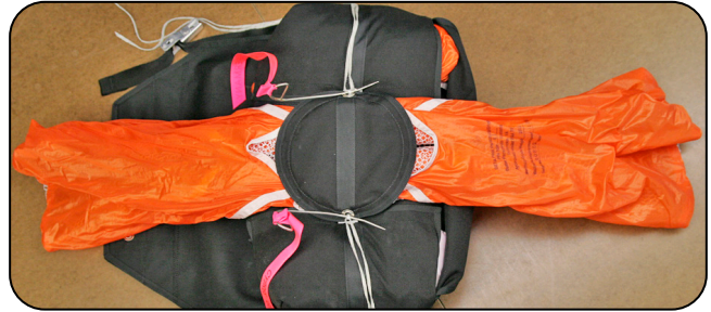
10.17 Folding the pilot chute material.
