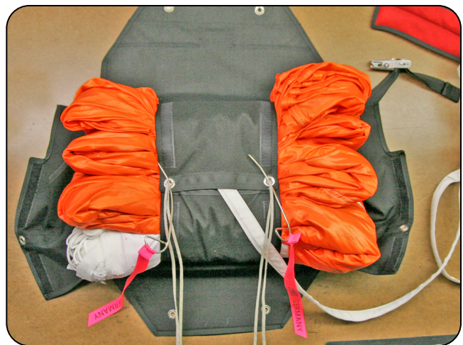
10.8 Closing the top staging flap.
