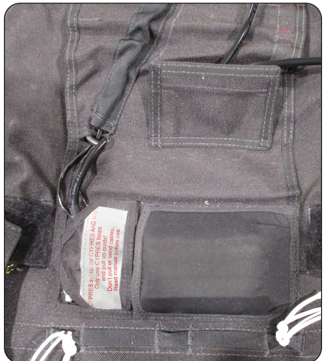
7.6 Stowing the control processor cable.
