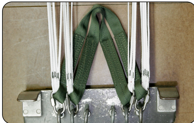
9.2 Installing the rear cross connector.
