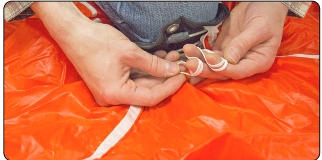
9.14 Clearing the center line.
