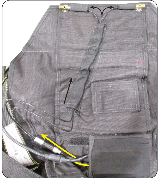
7.2 Stowing the cutter wires.
