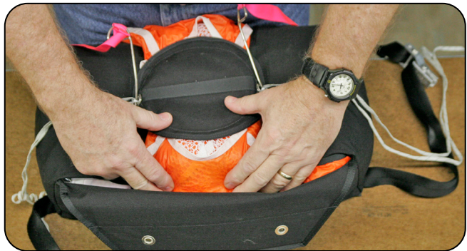
10.18 Folding the pilot chute material.
