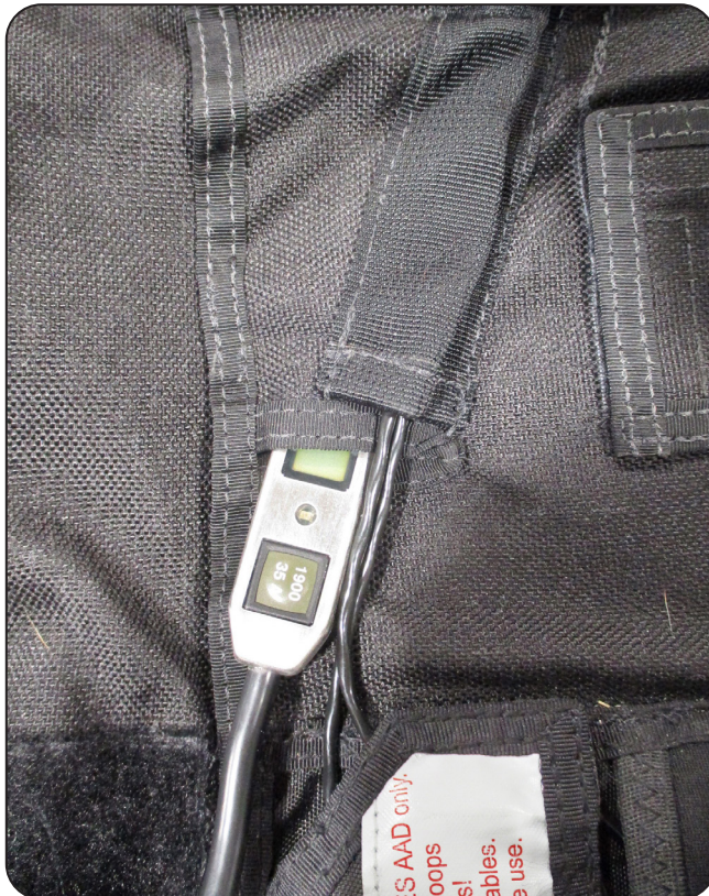
7.4 Routing the control cable.
