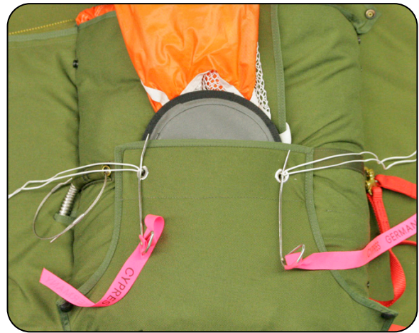
7.22 Closing the left container flap.
