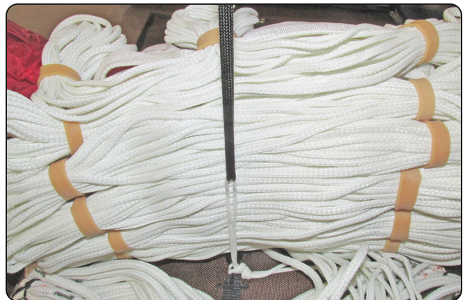
7.7.1 Closing loop comes straight up.
