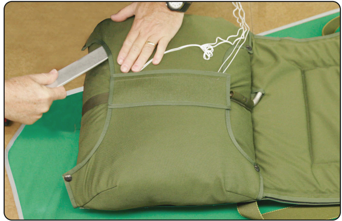
7.25 Dressing the container.
