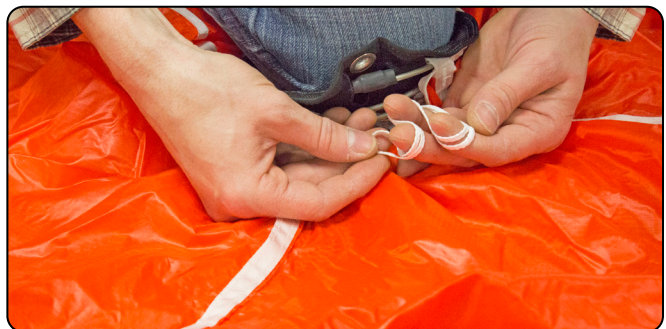
7.16 Clearing the center line.
