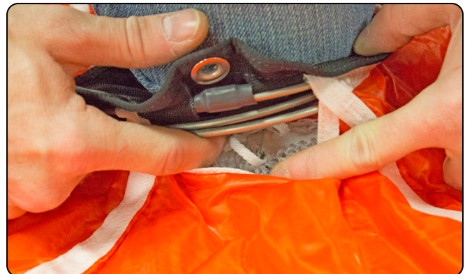
7.17 Folding and stowing the center line.
