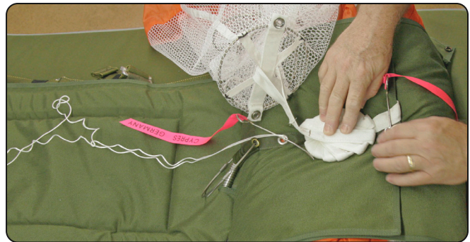
7.13 Stowing the pilot chute bridle.
