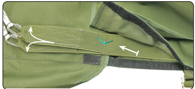
7.3 Tacking the risers.
