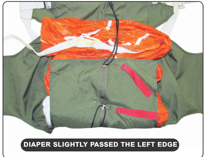
7.11 Closing the bottom flap.
