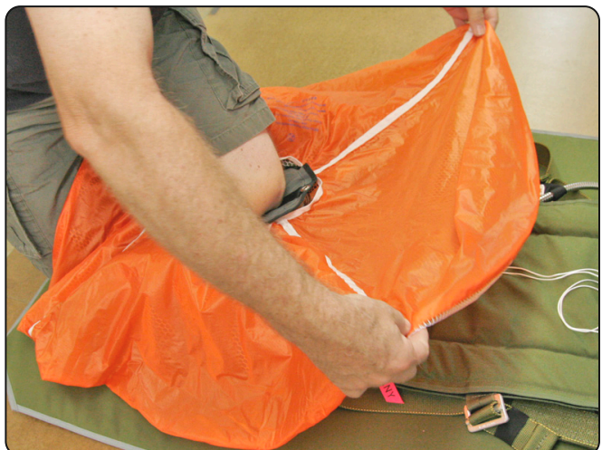
7.15 Compressing the pilot chute.
