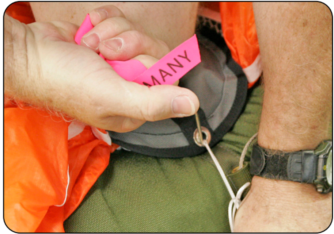
7.19 Pinning the pilot chute.
