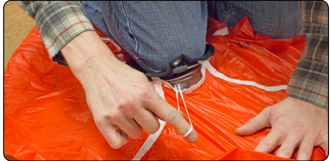
7.16 Clearing the center line.
