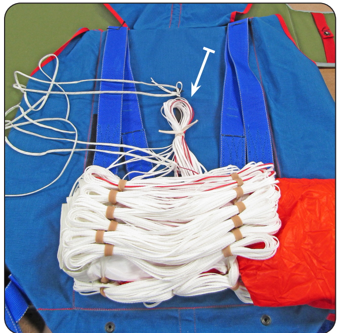
7.4 Tacking the risers.
