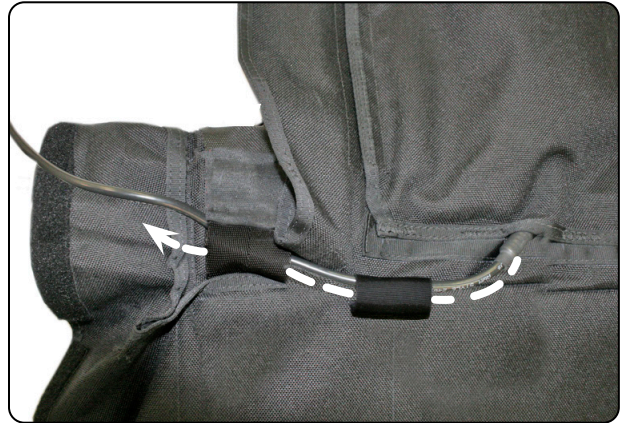
6.1.2.1 Routing the control unit cable.
