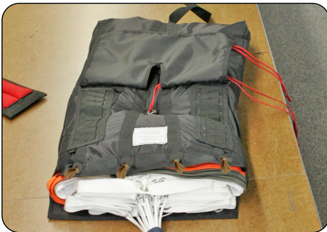
7.4.5 Folding the canopy into the deployment bag.
