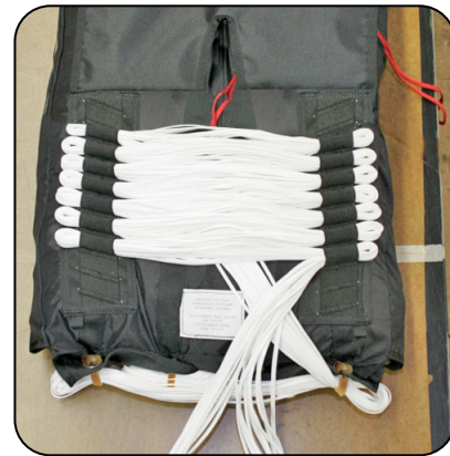
7.5.3 Stowing the suspension lines.
