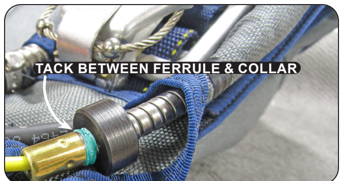
6.1.1.4.2 Installing the arming cable housing with the Dual Mode option.
