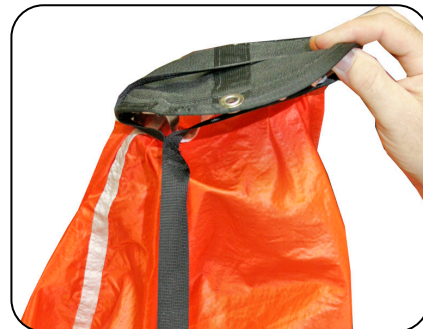
7.2.12 Threading the channel bridle.
