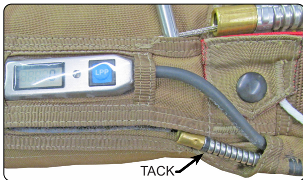
6.1.1.4.1 Installing the arming cable housing.
