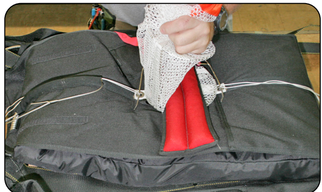
7.6.10 Securing the pilot chute.
