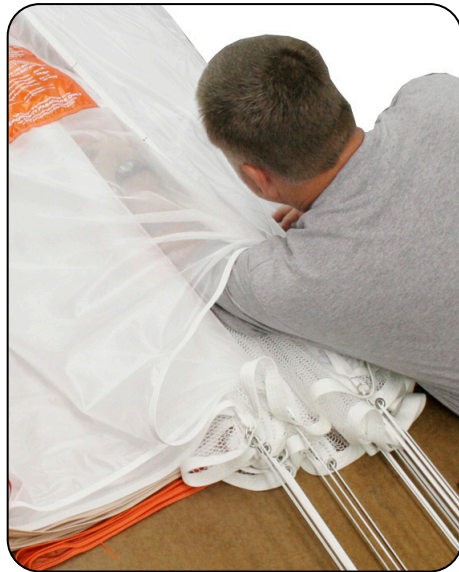
7.3.3 Stowing the slider.
