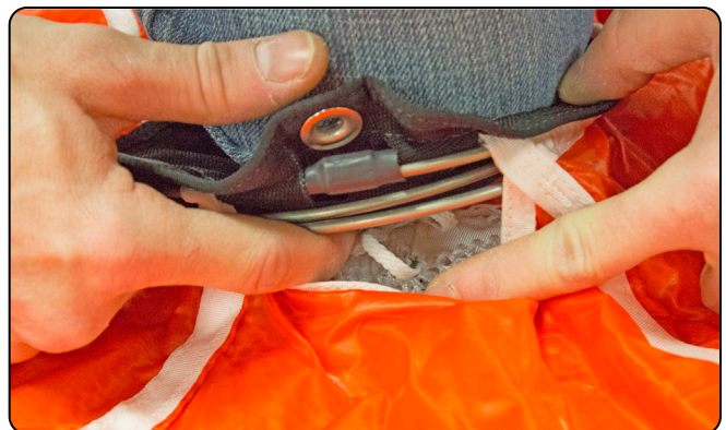
7.6.13 Folding and stowing the center line.
