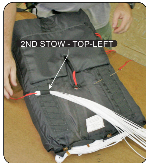
7.5.2 Stowing the suspension lines.
