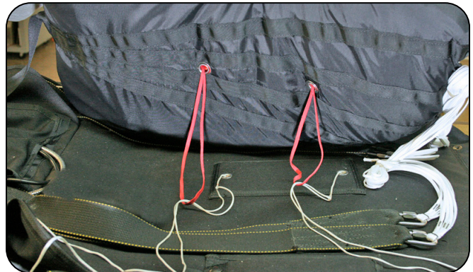
7.6.5 Threading the pull-up cords.
