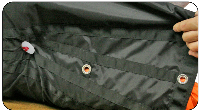
7.4.2 Folding the canopy into the deployment bag.
