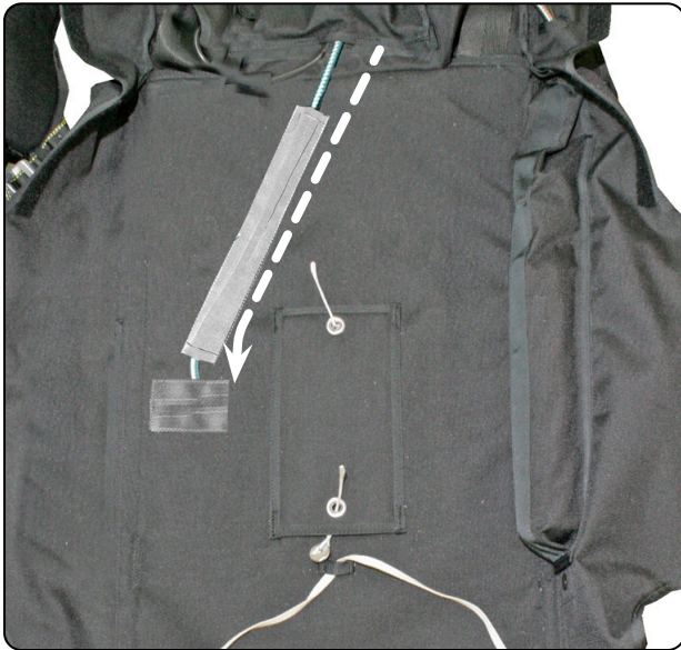
6.1.2.3 Installing the arming cable housing.
