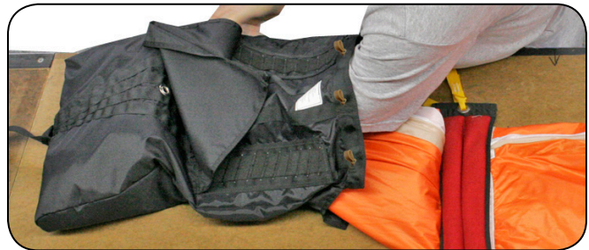
7.4.2 Folding the canopy into the deployment bag.
