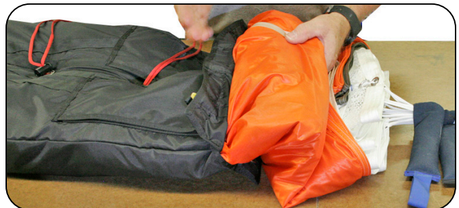
7.4.5 Folding the canopy into the deployment bag.
