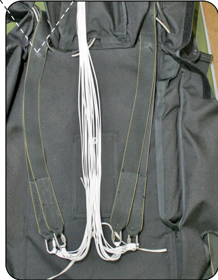
7.1.13 Tacking the risers.
