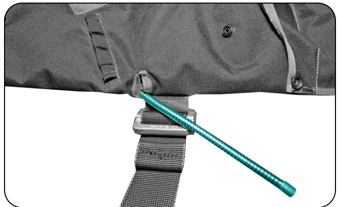
6.1.2.3 Installing the arming cable housing.
