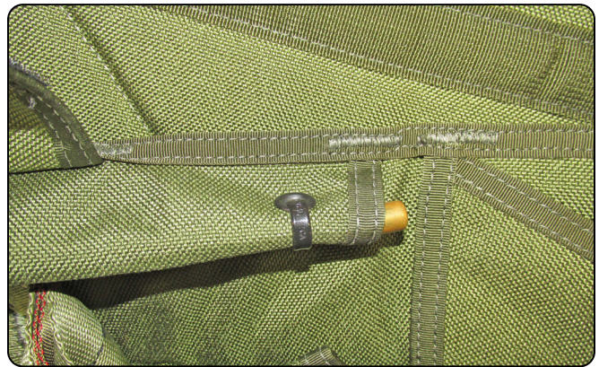
6.2.6 Installing the cable tie.
