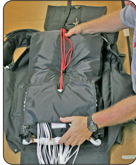
7.6.1 Placing the bag.
