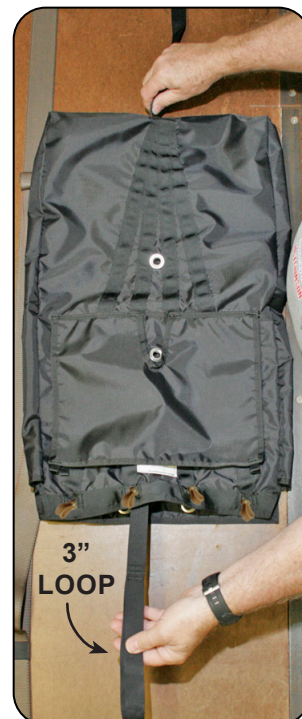
7.2.8 Pilot chute bridle through the deployment bag.
