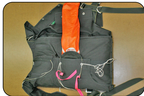
7.6.17 Closing the left container flap.
