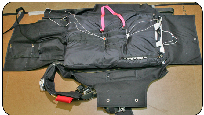
7.6.6 Securing the pull-up cords.
