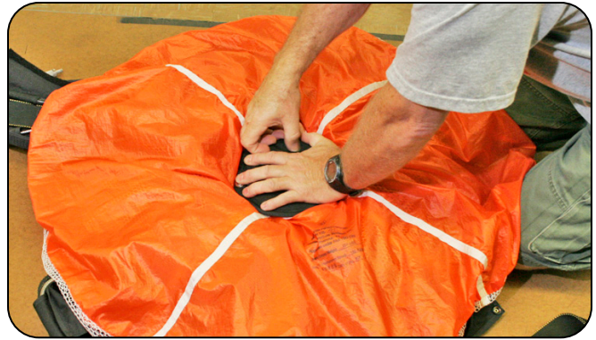
7.6.11 Compressing the pilot chute.
