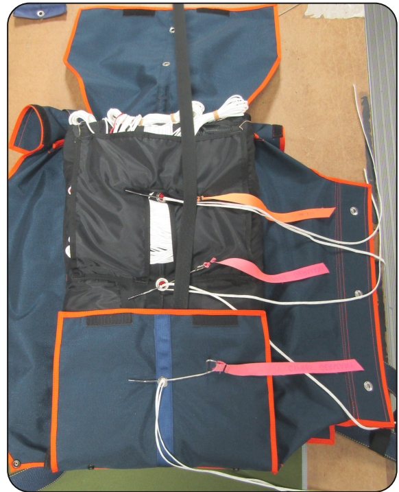
7.3.6 Closing the bottom flap.
