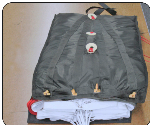
7.1.4 Folding the canopy into the deployment bag.
