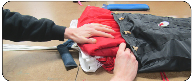
7.1.3 Folding the canopy into the deployment bag.
