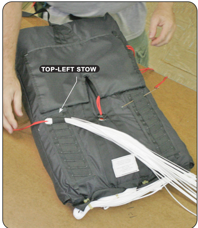
6.2.2 Stowing the suspension lines.
