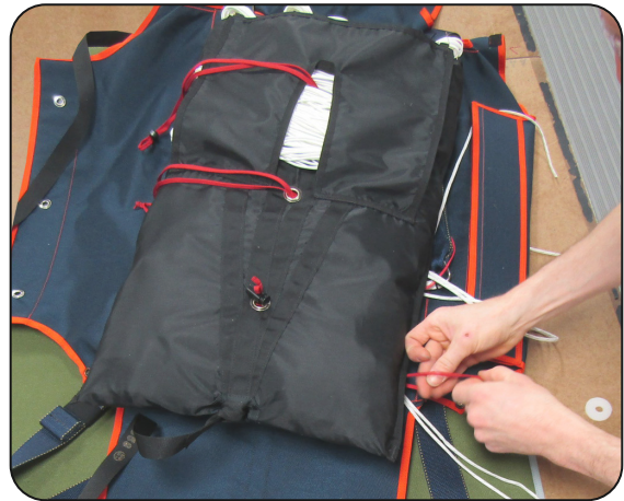
7.3.4 Threading the pull-up cords.
