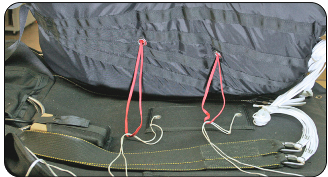
6.3.5 Threading the pull-up cords.
