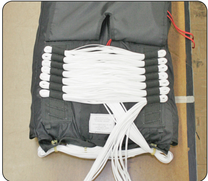
6.2.3 Stowing the suspension lines.
