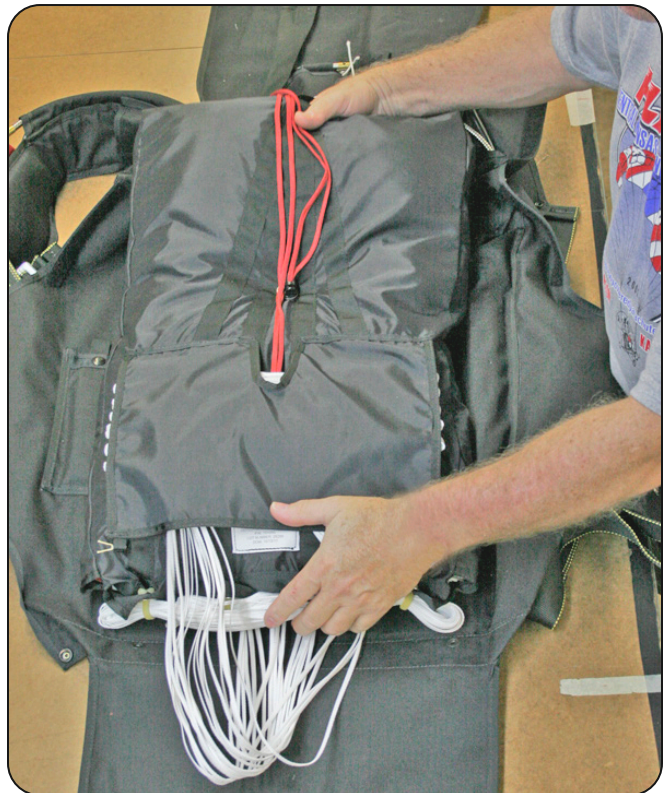
6.3.1 Placing the bag.
