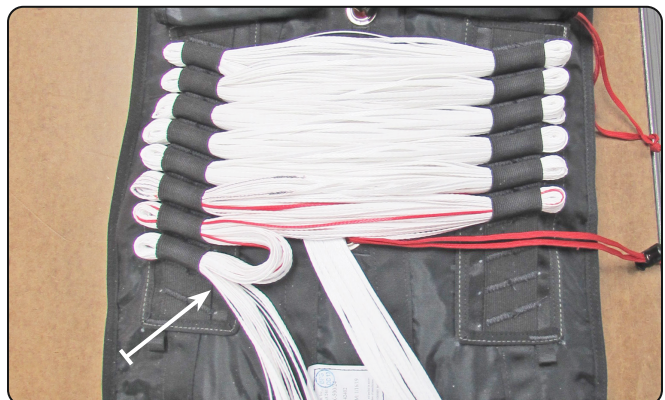
6.2.3 Stowing the suspension lines.
