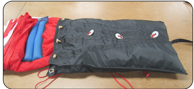
7.1.3 Folding the canopy into the deployment bag.
