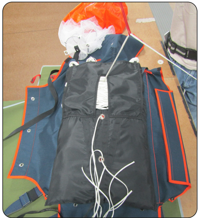
7.3.4 Threading the pull-up cords.
