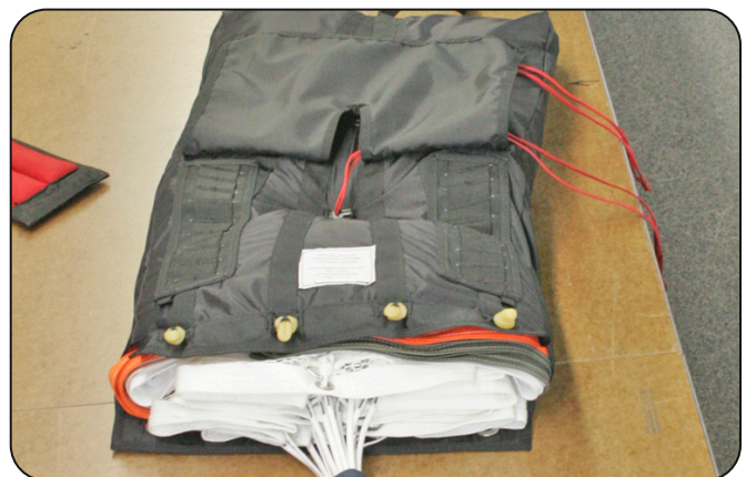
6.1.4 Folding the canopy into the deployment bag.
