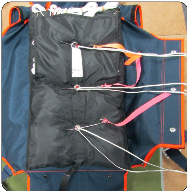
7.3.5 Securing the pull-up cords.
