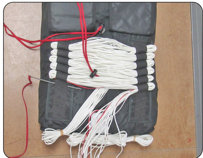
7.2.4 Stowing the suspension lines.
