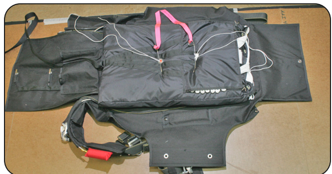
6.3.6 Securing the pull-up cords.
