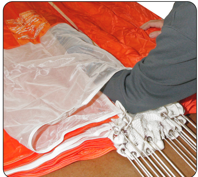
9.3 Stowing the slider.
