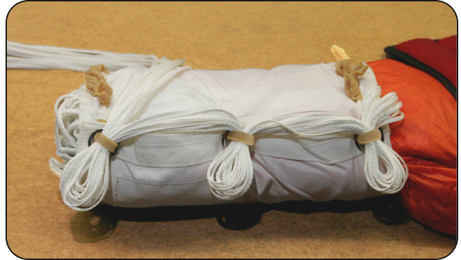
10.6 Closing the remaining locking stows.
