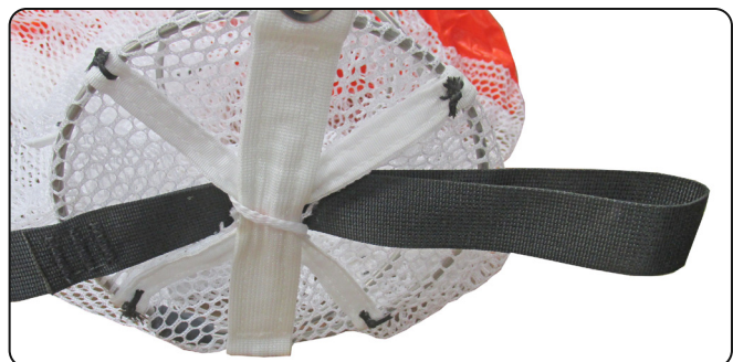
8.3 Threading the bridle.
