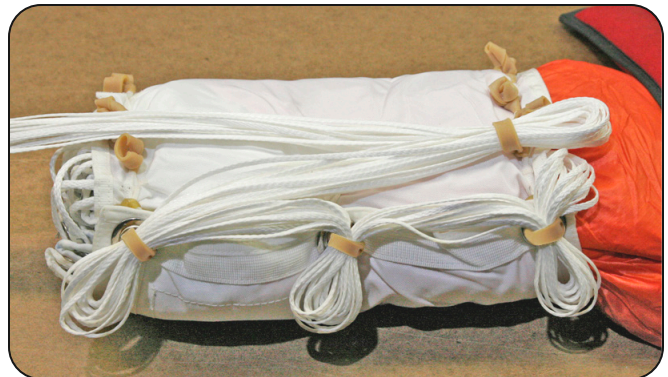
10.6 Closing the remaining locking stows.
