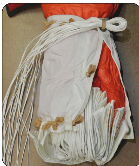
10.4 Closing the first locking stow.
