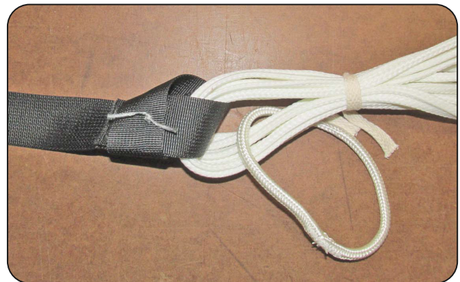
8.1 Bridle installation onto the apex.
