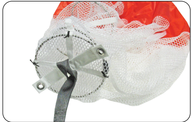
7.6 Installing the pilot chute.
