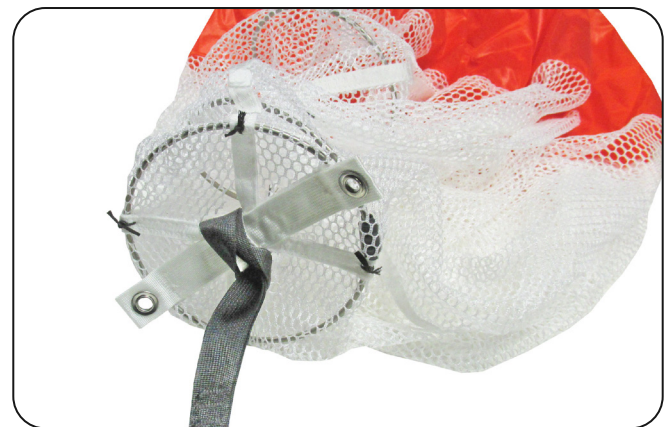
8.4 Installing the pilot chute.
