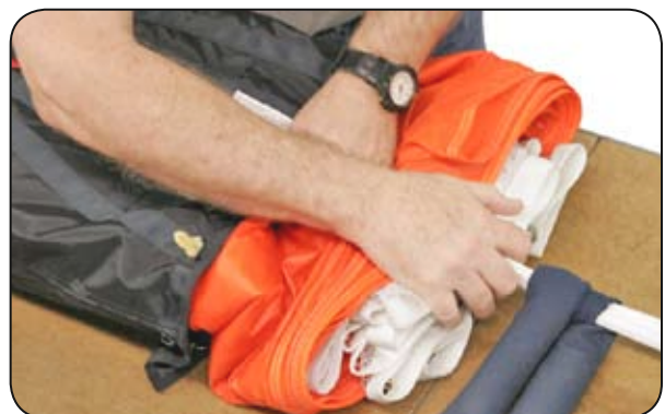
7.6 Inserting the skirt of the canopy.
