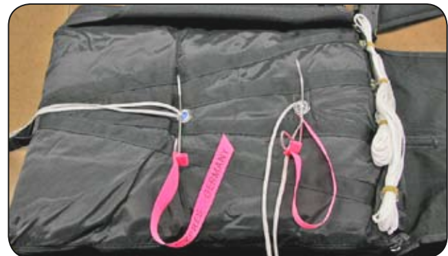
9.5 Pulling the cords through the deployment bag.
