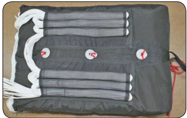
8.3 Stowing the suspension lines.
