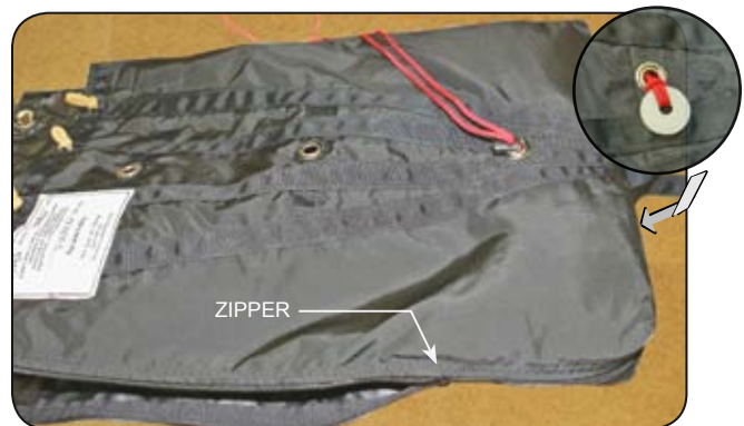
7.4 Installing the locking pull-up cord.
