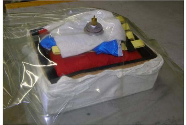
A2-3) The fixture and parachute are "bagged".
