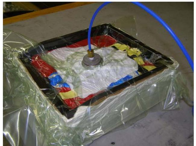
A2-5) The parachute is sucked down to the rigger's satisfaction and is ready to go into the oven to bake.
