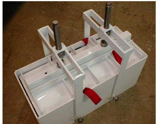
A1-5) Packing fixture with parachute compressed to proper point to soak and relax.
