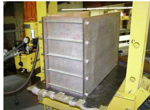
A3-4/5/6) The shell is placed into the fixture, the side and end plates are closed up, then tightened down with the cross bolts.
