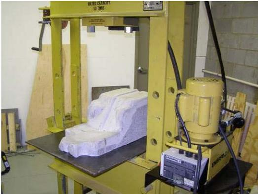
A3-2) The concrete mold to support the shell evenly
