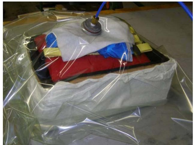
A2-4) The vacuum port is placed in the film.
