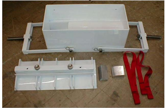
A1-3) Fabricated aluminum packing fixture (empty)
