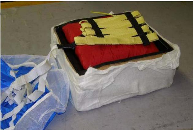
A2-2) The parachute which is hand packed into a shaped deployment bag is placed into the fixture.
