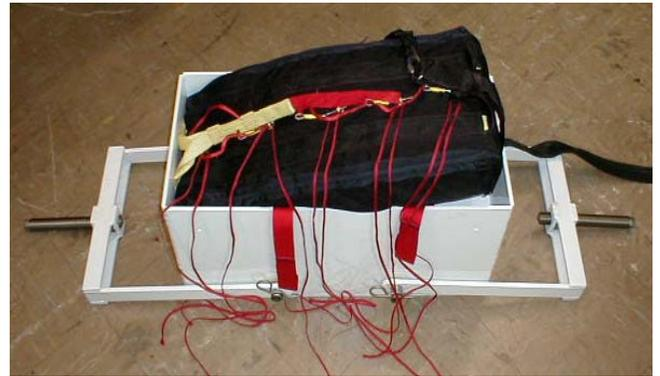
A1-4) Packing fixture with d-bag partially fitted.
